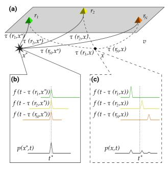
**Figure 3.** Back-projection general concept: (a) a simplified scheme of receivers and travel-times precomputed using ray-bending in the proper velocity model for two points of a study region; (b) back-projection to the actual location of the seismic event; (c) back-projection to the virtual source point with incorrect travel-times.
