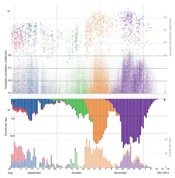
**Figure 10.** The MF-based catalog of lower-energy events in comparison with cluster analysis results for the BP-based catalog containing most-energetic earthquakes (in pale colors): (a) CCs for both catalogs (note that these are not the same type); (b) time distribution of the events' daily amount.
