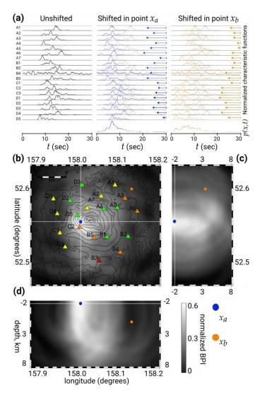
**Figure 4.** Example of the BP detection procedure for a high-energy LP event on Gorely: (a) signal envelopes (CFs) shifted according to precomputed travel-times; (b) horizontal, and (c,d) two vertical slices of 3-D BPI snapshot for a time of local maximum in detector function.
