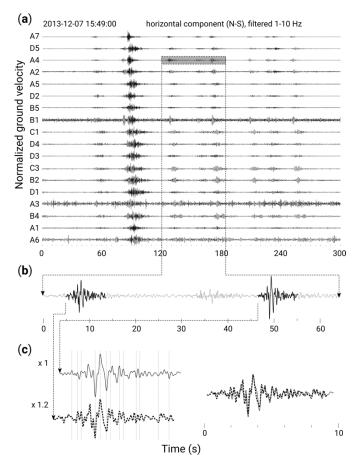
**Figure 2.** Example of LP swarm on Gorely: (a) 5-minute horizontal component records of 18 temporary stations; (b) zoom on representative LP signals at station A4; (c) close comparison of two waveforms.
