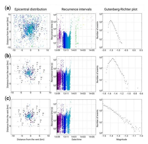
**Figure 5.** Results of applying the BP detection algorithm to Gorely data: (a) detections acquired using records of five temporary stations which functioned nine months; (b) same for 18 stations working during the four starting months, when degassing activity was exceptionally strong; (c) filtered detections obtained with 18 stations, which follow Gutenberg–Richter law and constitute BP-based catalog.
