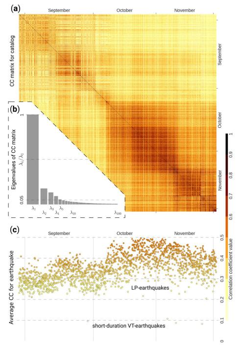
**Figure 7.** Similarity assessment of earthquakes from the BP based catalog: (a) waveform CC matrix; (b) first 100 eigenvalues of the matrix—sorted and normalized; (c) mean average similarity for each earthquake inside the catalog.
